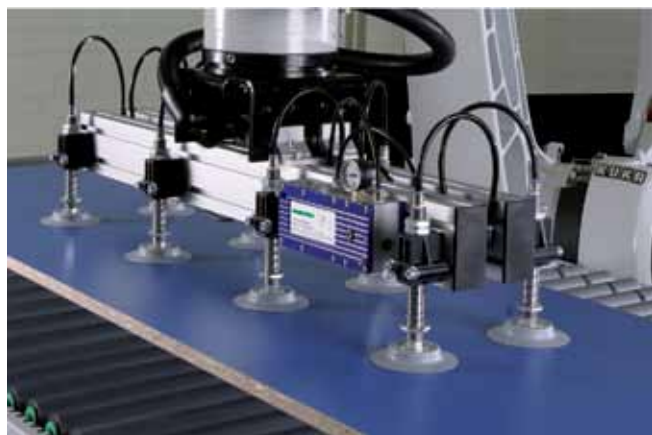
Suction plates. NSPUX being used for handling coated chipboards
