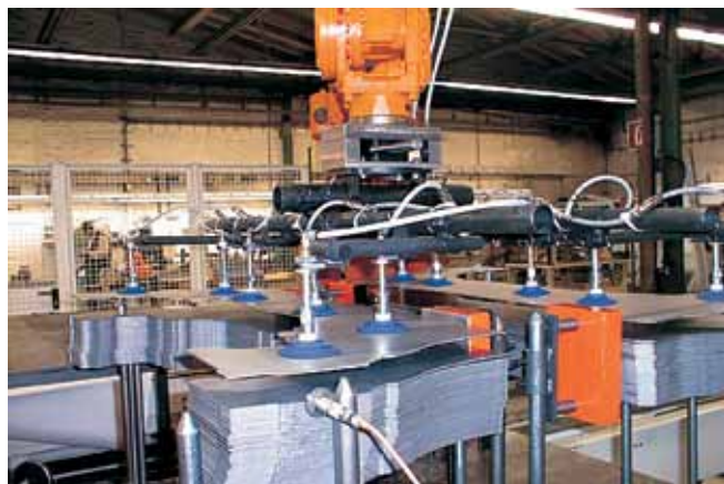
Mounting example spring plungers NFSTE
