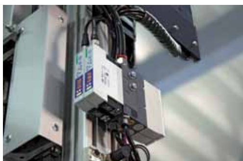
Centralized vacuum generation by means of compact ejectors NSCPI
