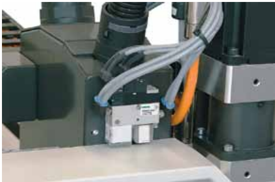
Central vacuum generation by compact ejectors NSCPM
