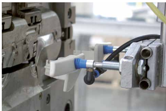
Bellows suction cups NFSGX being used for handling hot plastic parts
