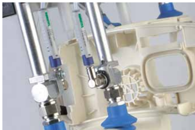
Decentralized vacuum generation by means of inline ejectors NtSLP for handling plastic injection molded parts
