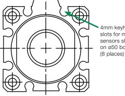
4mm keyhole slots for mounting sensors shown on ø50 bore
