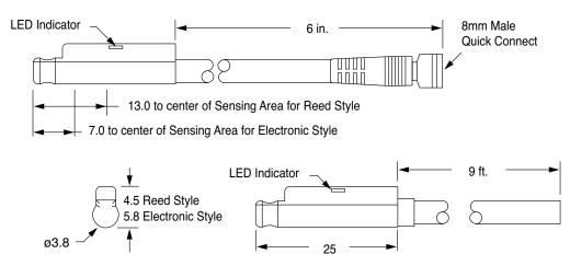
All sensors feature surge suppression, polarity protection, LED indicator, and extremely fast switching speeds.
