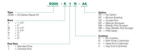
NOTE: Options listed are ones that apply to a repair kit only. Model number is set up to use option code supplied with original cylinder or with any above.
