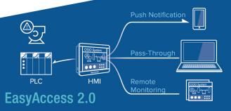
The HMI is not just for operating machines, collecting and managing data, but also plays a key role in IIoT as a Communication Gateway. The data in the device connected to HMI can be published to IIoT system.
