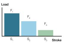
Fm= Equivalent dynamic axial load in NF1, F2... Fn= Load exerted over a segment of travelled<br/>distance sn
