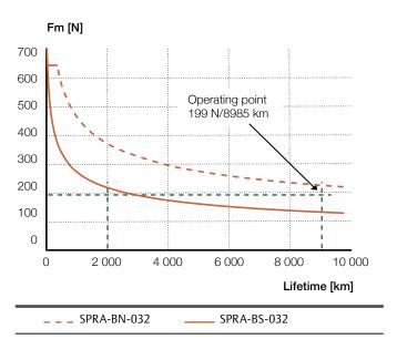
The operating point is below the dashed line. The SPRA-BN-032 is the smallest linear unit for this application which fulfills the requirements.
