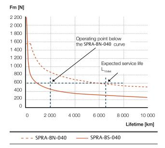
The operating point is below the SPRA-BN-040 curve. It is the smallest linear unit which fulfills the requirements. The expected service life is almost 6500 km.
